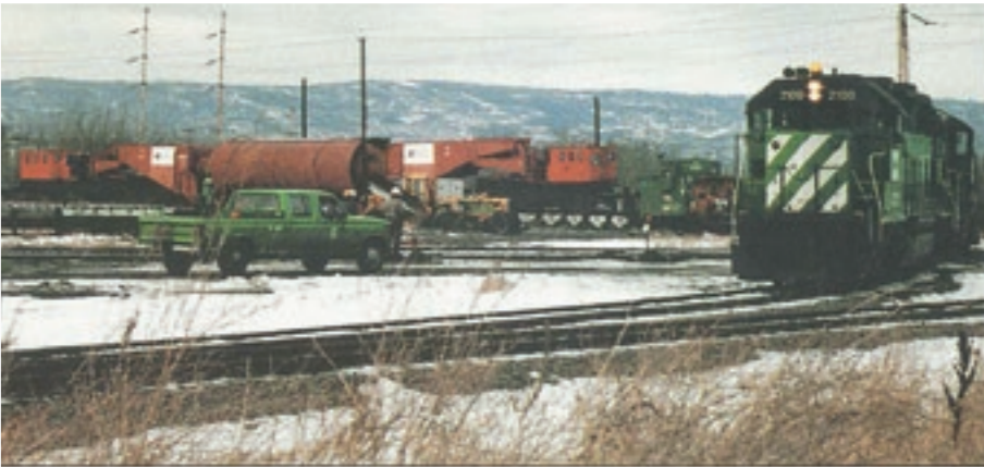
(Above) The completed train moves around a curve in the former Burlington Northern Railroad Yard in Superior, Wisconsin. The Schnabel Car was used in the 1,000-mile move between Duluth and Regina, Saskatchewan. (Below) One of the reactor units leaves the Clure Terminal at the start of its 10-day, one-way trip.
