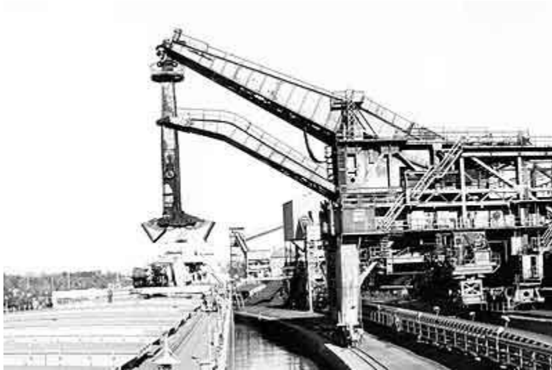
The Hulett Unloader, invented in 1899, revolutionized the discharge of iron ore at Lake Erie ports. In this photo, the John G. Munson is unloaded at Lorain, Ohio. (Lake Superior Marine Museum Association Archives, Lake Superior Maritime Collection at University of Wisconsin-Superior, USX Great Lakes Fleet photo)
