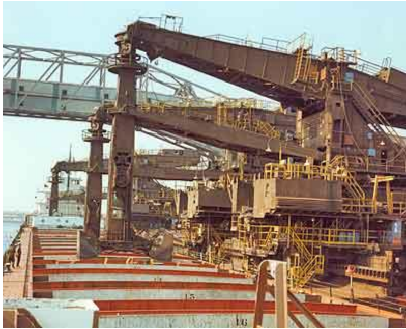
A massive Hulett Unloader discharges iron ore from the William A. Irvin at a Lake Erie port. (SS William A. Irvin Museum Collection, Duluth Entertainment & Convention Center)
