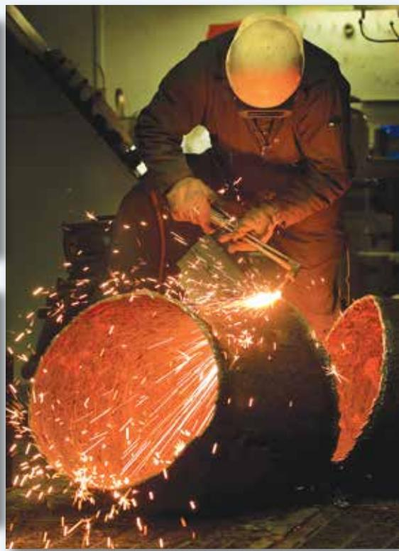
A pipefitter cuts an old ballast pipe section being replaced in a freighter.
