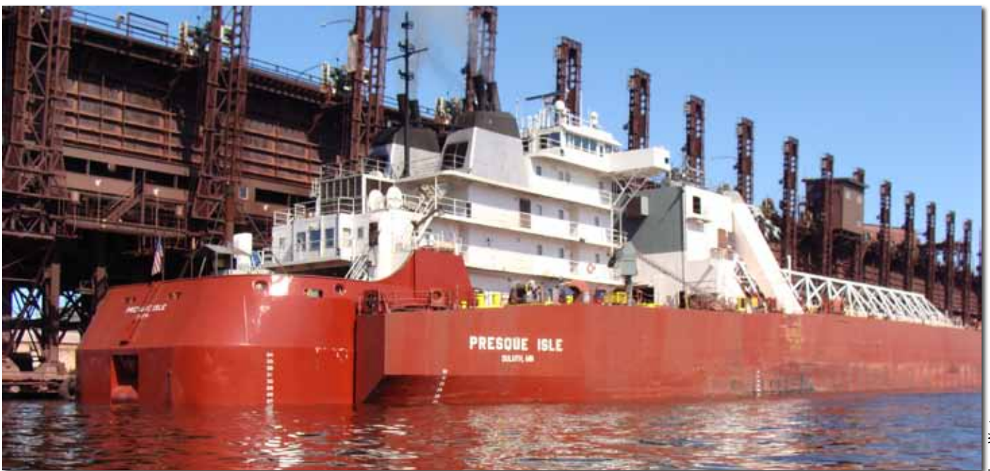
This view of the Presque Isle clearly illustrates her tug (aft) barge (fore) configuration.
